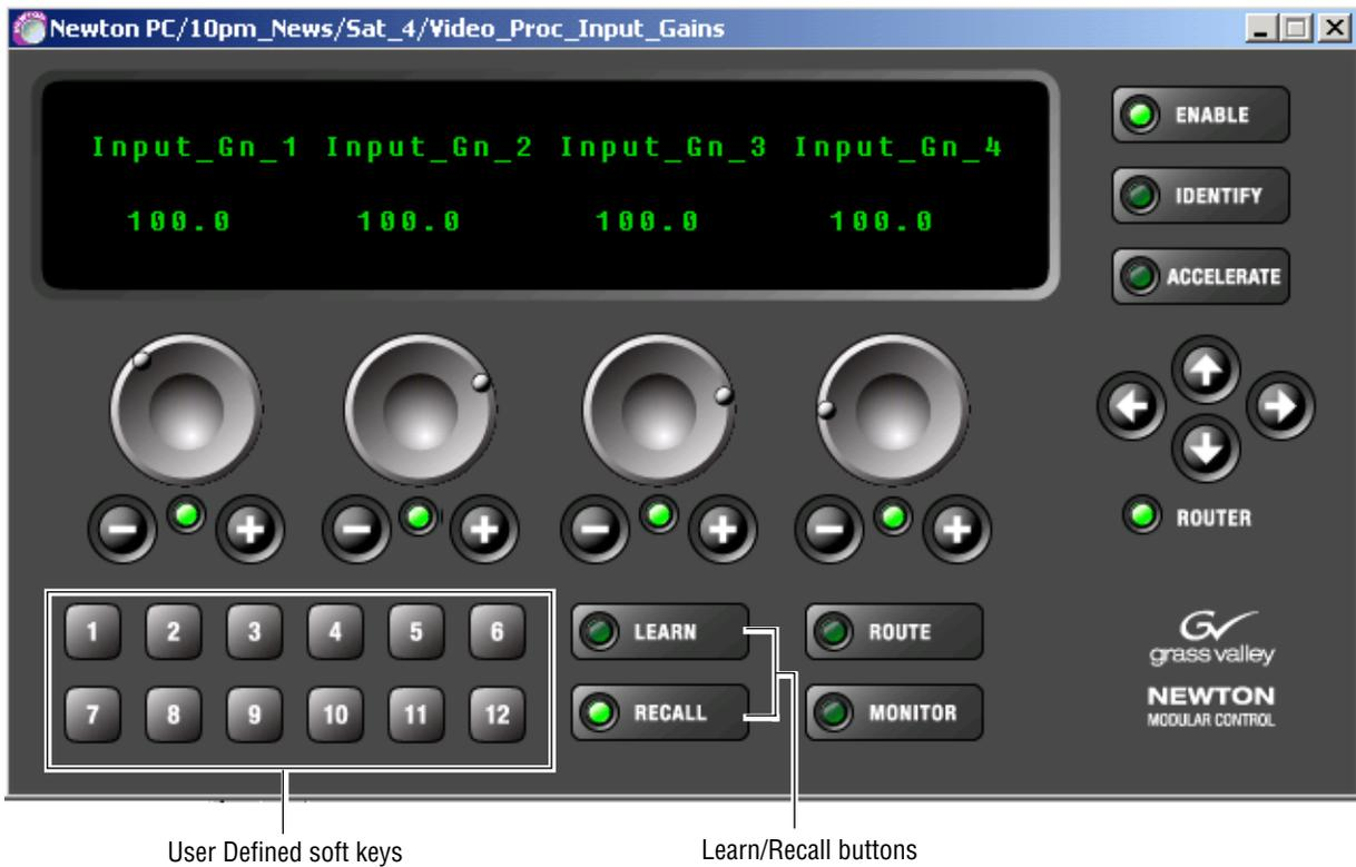
Figure 82. Rack Mount Panel Soft Keys and Learn/Recall Buttons
