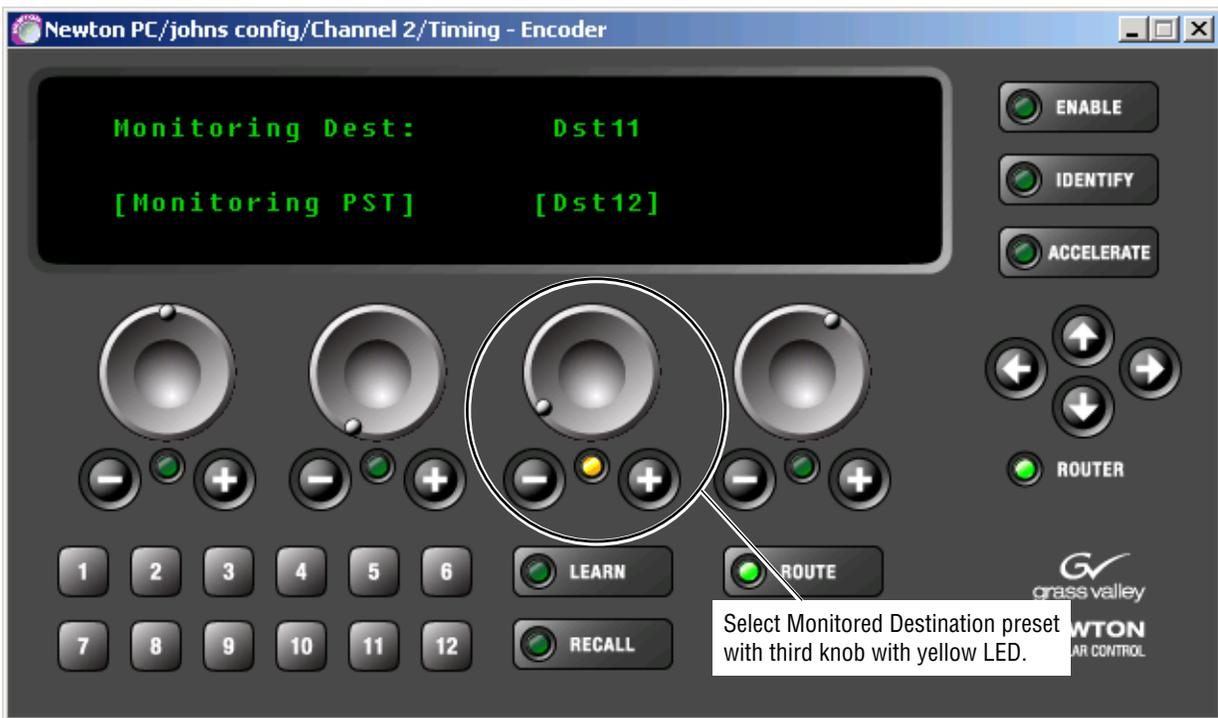
Figure 76. Monitored Destination Display on Rack Mount Panel
