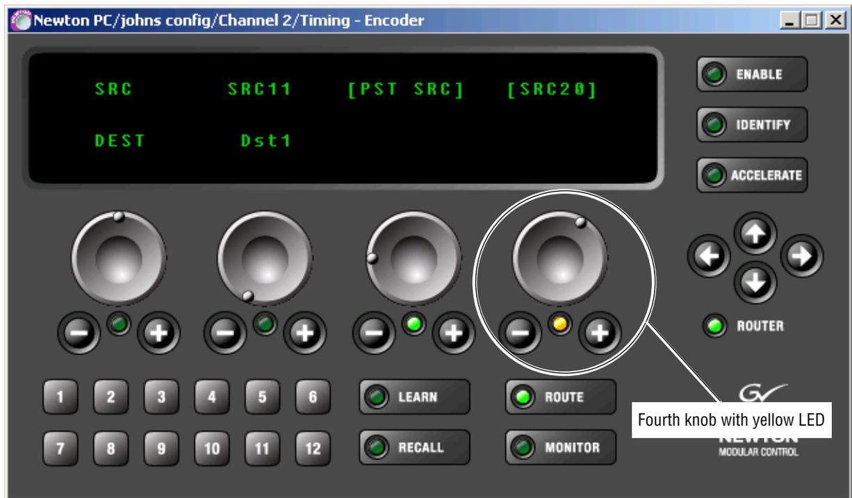
Figure 71. Source Select Mode on Rack Mount Panel
